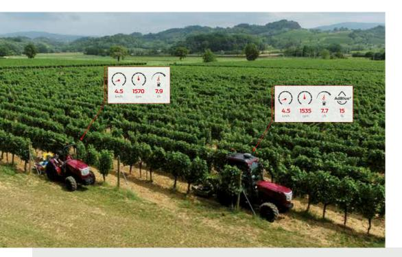
by checking parameters like speed, engine take informed decisions. hours and RPMs, fuel and AdBlue levels, average consumptions and work progress.
