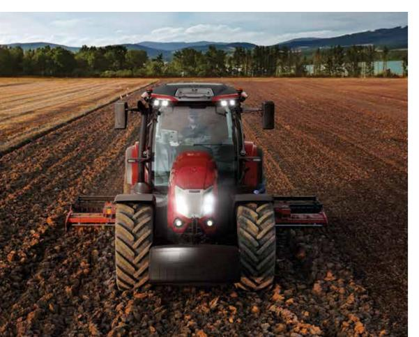
The **X8** tractors are powered by new FPT NEF 67 6.7-litre, 6-cylinder turbo intercooled engines with multivalve technology and electronic common rail injection system. The eVGT variable-geometry turbocharger provides optimum engine performance and fast response to load changes. The maximum torque is available already at 1400 rpm. The HI-eSCR2 exhaust gas aftertreatment system ensures compliance with Stage V emissions regulations.
