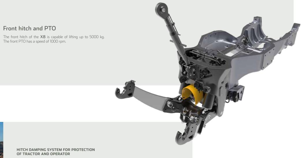
The **X8** is designed to handle heavy-duty implements with maximum efficiency. During headland turns and transport operations, heavy implements generate shock loadings. Both the rear and front hitch of the **X8** feature a damping system with two nitrogen charged accumulators that minimises tractor pitching when travelling with raised implements, making for a smoother and more comfortable ride.
