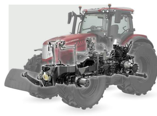
The **X8** tractors feature a closed centre hydraulic system with variable displacement pump. This means that the pump always delivers exactly the quantity of oil that the system requires, thereby eliminating unnecessary power waste. The system supplies 160 l/min to the hitch and remote valves and 115 l/min to the electronic steering system, allowing for simultaneous operation of all hydraulic functions. A pump with up to 212 l/min flow rate is also available to provide high-flow capability.
