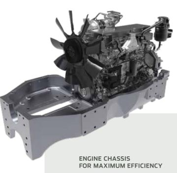
The FPT NEF 67 engine is located within a rugged chassis and mounted on silent block rubber mounts to isolate both cab and transmission from vibrations and noise. This solution moves the tractor's centre of gravity forward, improving the vehicle's balance while increasing traction.
