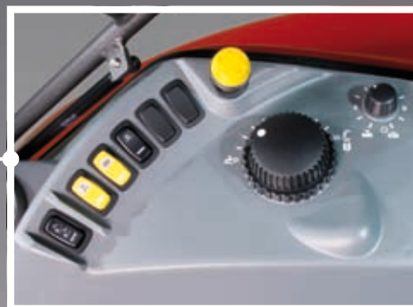
Console. The PTO switch is installed on the driver's right.
