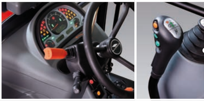
The controls. Left. The lever on the steering wheel that operates the hydraulic reverse shuttle. Reverses any gearshift gear without use of the clutch pedal. Right. The lever of the T-Tronic gearshift which engages 3 Powershift ranges (H-M-L) by means of the green buttons.
